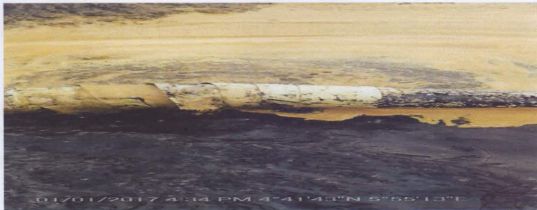
Flow line exposed but cause of spill not determined due to high pressure of Gas.
